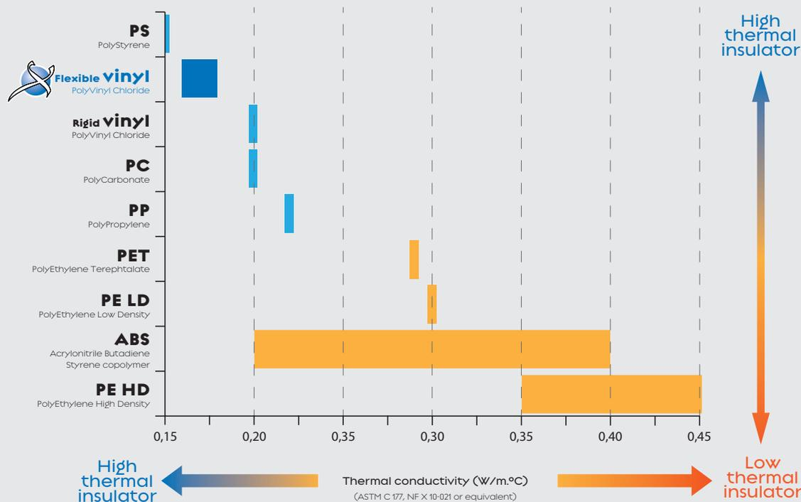
How to compare energy flow lost by thermal conduction through different materials?
