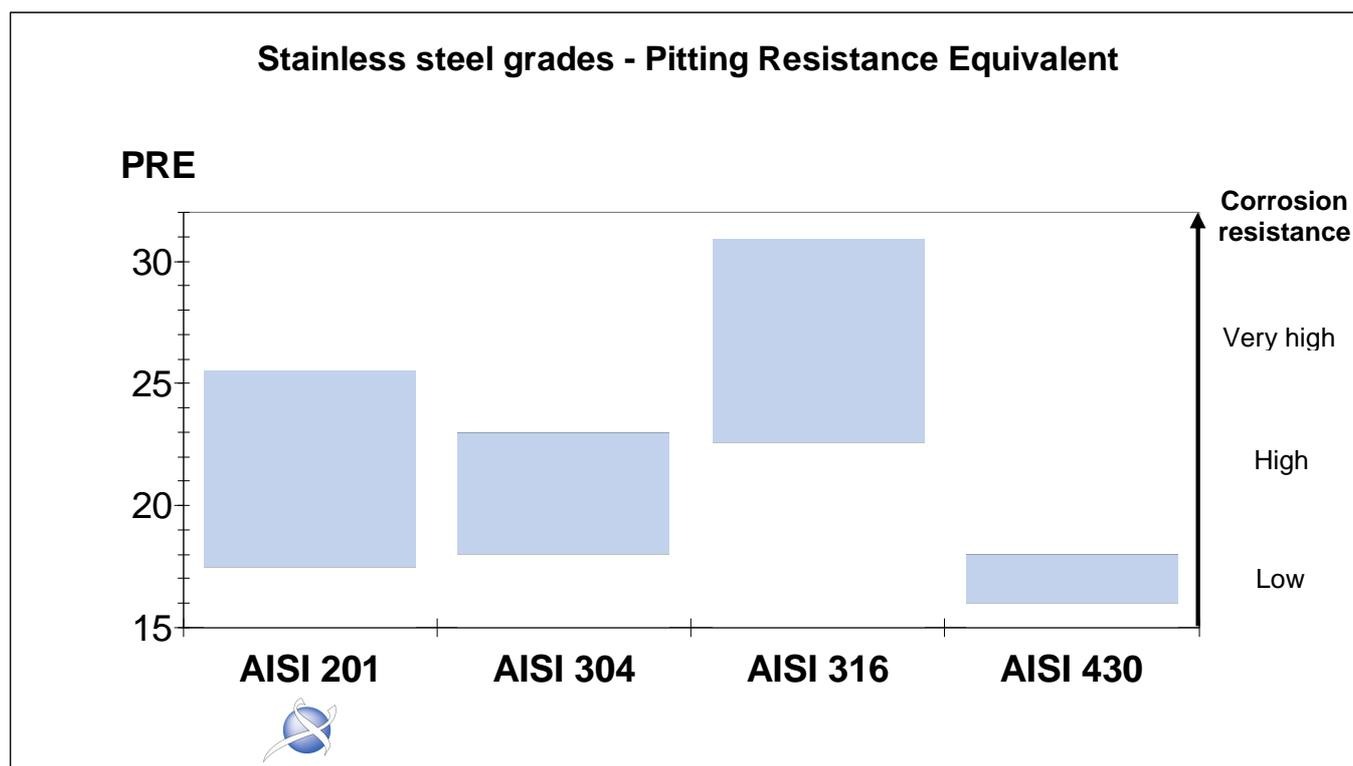
AISI 201 & 304 have comparable high corrosion resistance. They can be used in aggressive environment and are suitable for food process plant. Their corrosion resistances are perfectly adapted for industrial doors application.
